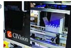
Pharmaceutical Kit Pack Inspection: CIVision inspects each kit to ensure that all elements are present and in proper position, and to verify UV codes (visible here as light blue dots).
